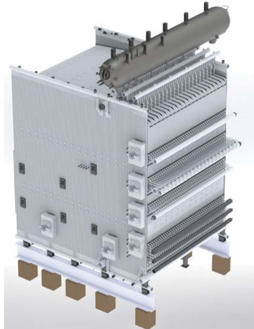
Bottom supported single drum boiler
